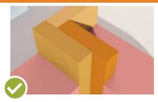
This is a three stud, or "California" corner which allows for max insulation coverage.
