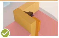
A two stud corner with a small nailing strip or drywall clips is a great alternative.
