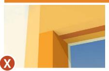
This header is NOT insulated resulting in a path for heat to transfer in or out of the home.
