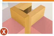
This corner framing does NOT accommodate insulation, reducing performance.
